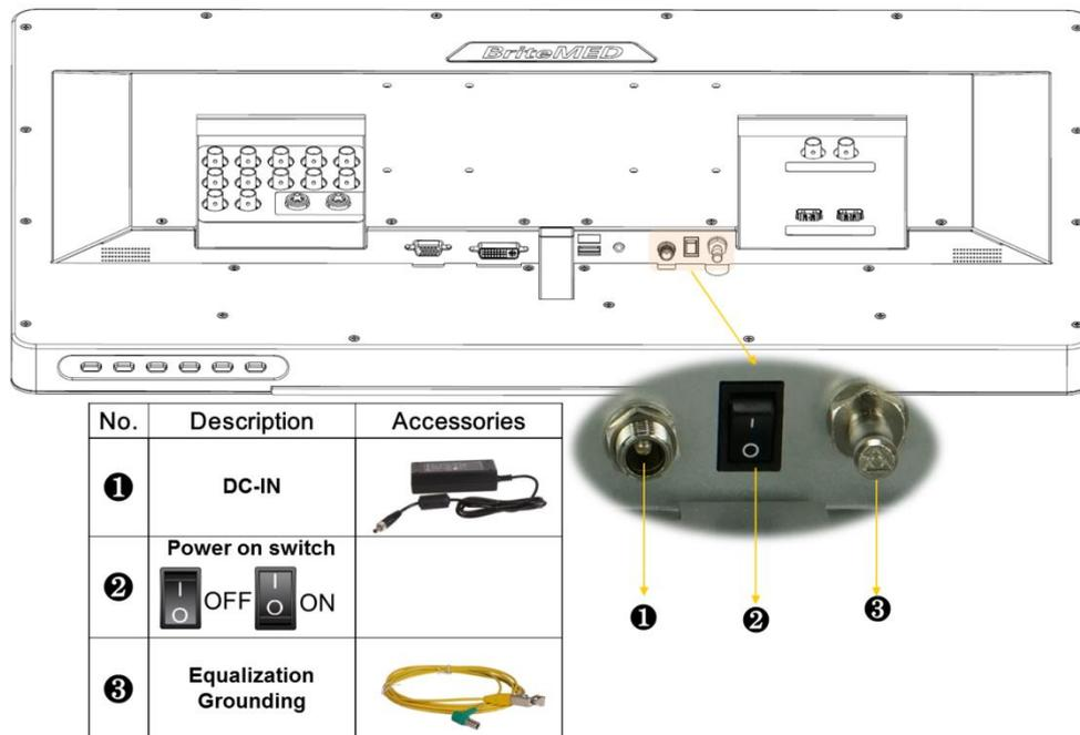
**Figure 3-2: Connecting the MMS-27C**
