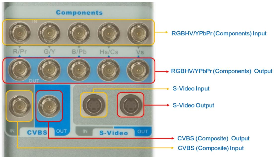
Figure 1-4: Analog Input and Output Connectors
