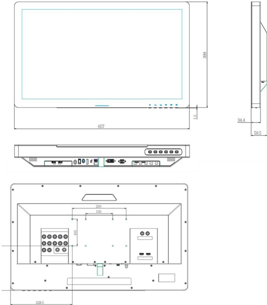
Figure 1-7: MMS-27C Dimensions (mm)
