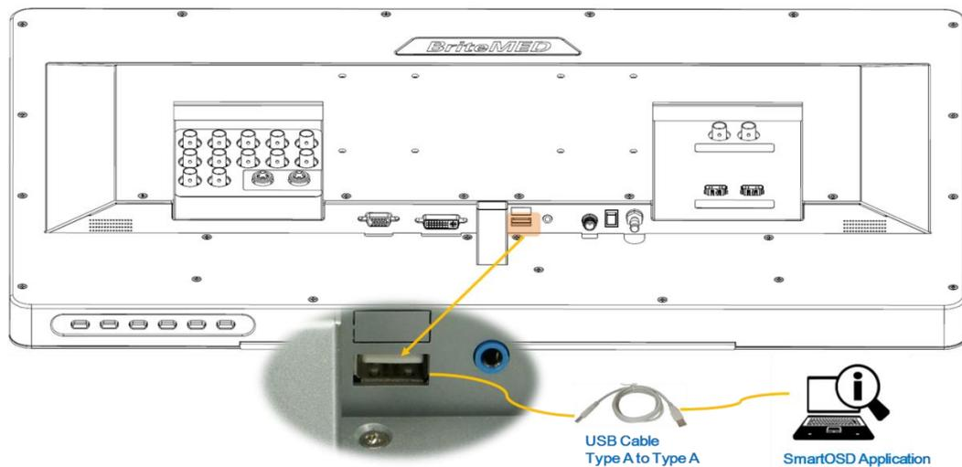
**Figure5-1: Using the USB Cable to Connect MMS-27C to a Computer**
